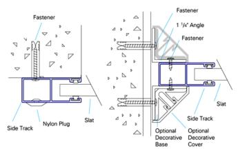
**Surface Mount**: Most common mounting application. Side track fits outside the rough opening.
